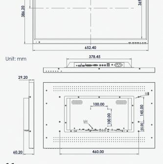
ROVER 28" PROFESSIONAL 4K LED CCTV MONITOR, 350CD/M<sup>2</sup>, METAL/STEEL PLATE CASE
