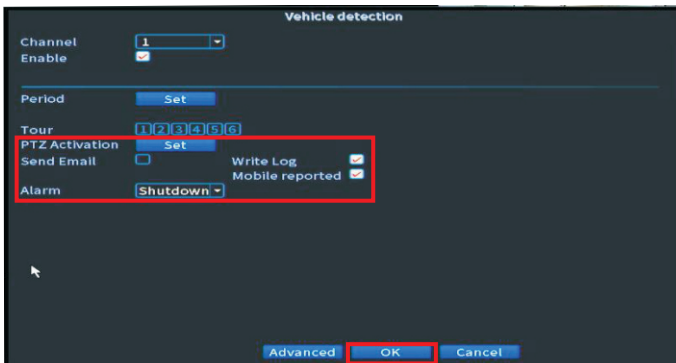
Figure 15. Set PTZ Activation, Send Email, Write Log, Mobile Reported, Alarm. Click OK button.
