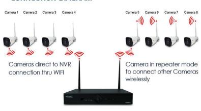
Can configure individual camera as a repeater to connect up to eight (8) cascading cameras connecting each other to work around 800 meters transmission distance but needs to check actual application and prior simulation to ensure effectivity.
