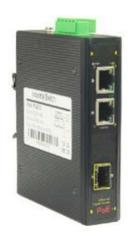
3-port Industrial Switch, with 2x 10/100/1000M Ethernet PoE ports and 1 gigabit SFP slot connecting devices like computers, switches, hubs, servers, etc. The Optical fiber SFP interface extends network transmission distance from 100m up to 20km. The Casing shell is made of aluminum extrusion. It is lighter, stronger, better resistant to corrosion, and electro magnetic interference, it ensures stability and security of Industrial Ethernet Switch. Uses standard DIN rail type installation method.
